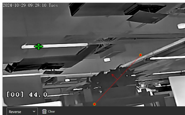
Figure 5-5 Set Single Line Crossing line
