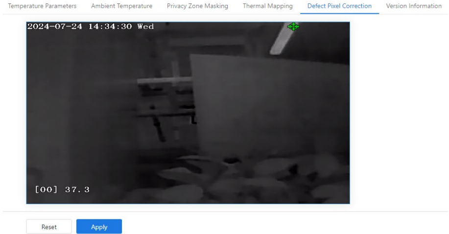
Figure 4-7 Recover Defect Pixel
