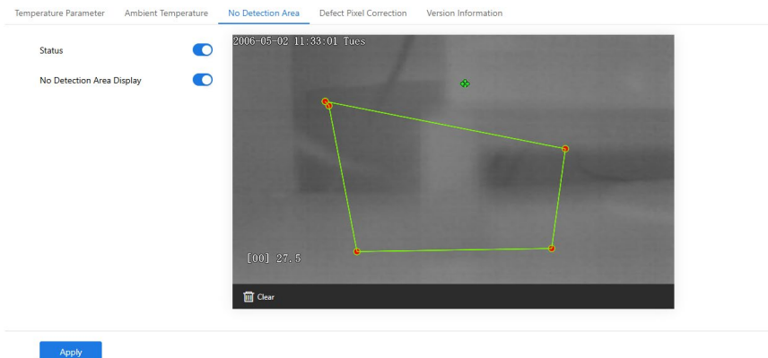
Figure 4-5 No detection area
